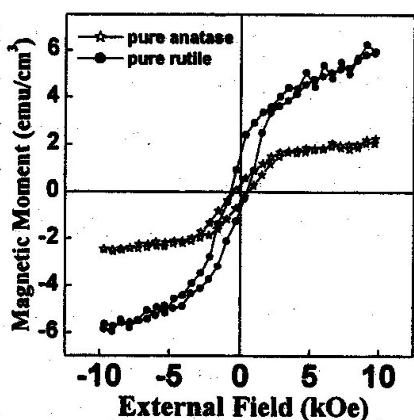
Figure 1. Results of magnetic hysteresis measurements on pure anatase and rutile films at room temperature.
